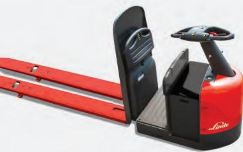
The ETR Series tractor series is designed to operate in indoor environments, towing trailers requiring up to 750 pounds maximum drawbar pull.
